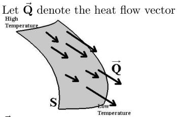
$\vec{\mathbf{Q}} \bullet \vec{\mathbf{n}} \, dS$  is cal/sec of heat flowing through a section of surface of area dS
