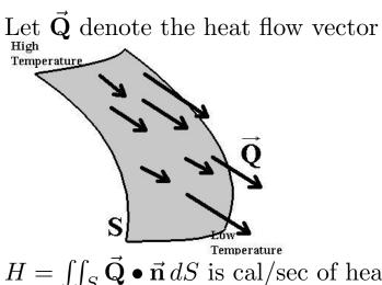
$H = \iint_{S} \vec{\mathbf{Q}} \bullet \vec{\mathbf{n}} \, dS \text{ is cal/sec of heat flowing through the entire surface } S$
