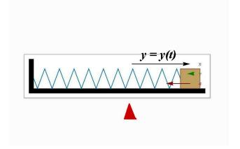
Hooke's Law: The force of the spring is proportional to the displacement of the object.
