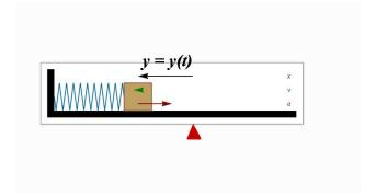
Resistive (damping) force is proportional to the velocity of the object
